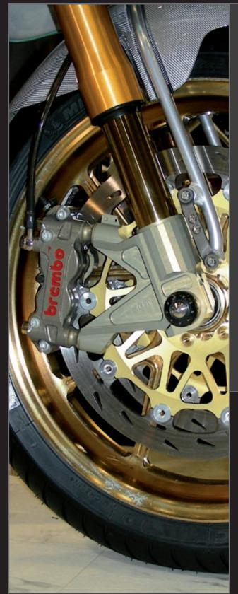
Moto Corse brake radial mounts are crafted by precision machine tools as shown, the caliper mount is "box" type precision tooled from single ERGAL 7075 solid piece.
